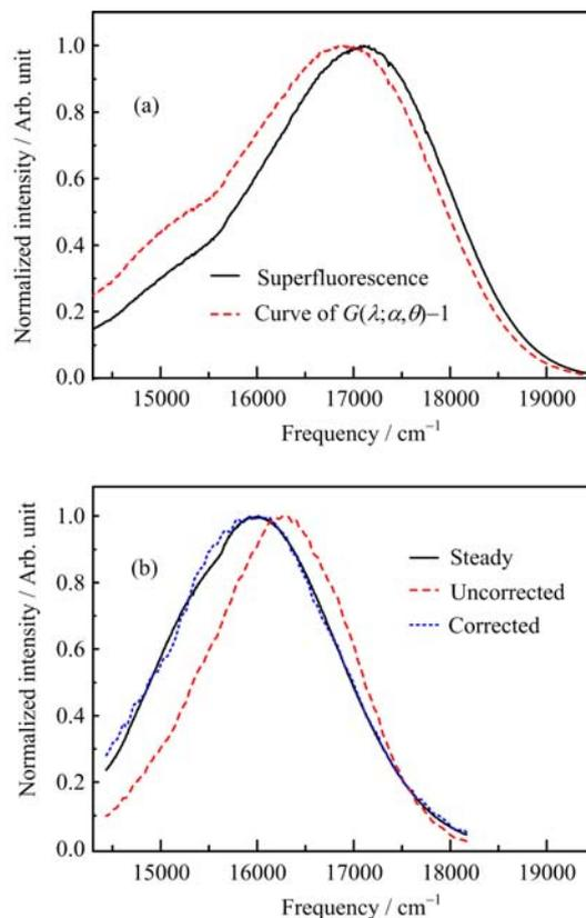
FIG. 1 (a) Normalized spectrum of parametric superfluorescence and normalized curve of  $(G(\lambda; \alpha, \theta) - 1)$ . (b) Comparisons between the DCM molecule steady fluorescence spectrum, corrected and uncorrected transient fluorescence spectrum at time delay of 36 ps.
