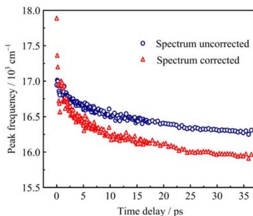
FIG. 2 Solvation induced dynamic Stokes shift obtained from transient fluorescence spectra with spectrum correction and without spectrum correction, respectively.
