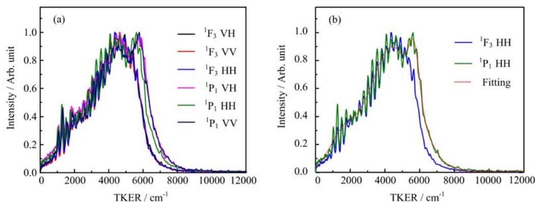
FIG. 2 (a) Total kinetic energy distributions for the  $S(^1D_2)+CO(X^1\Sigma^+)$  product channel from the photodissociation of OCS at 207 nm. (b) Comparison of TKER spectra in different intermediate states with the same polarization geometry. Fitted curves of the TKER spectra in the HH geometry with the  $^1P_1$  as resonant intermediate using three Gaussian functions are illustrated with red dot line.
