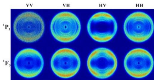
FIG. 1 Raw time-sliced ion images of  $S(^1D_2)$  products from the photodissociation of OCS at 207 nm.
