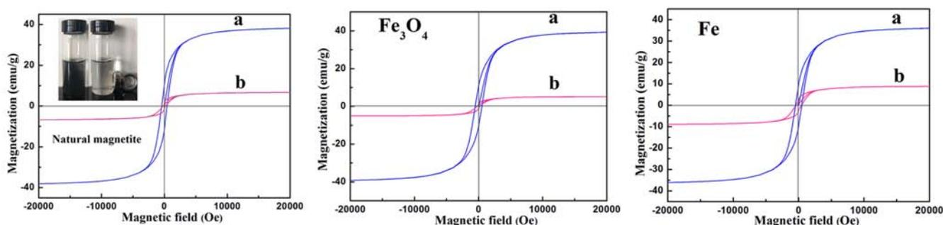
FIG. 4 The magnetic hysteresis loop of the  $\text{Fe}_3\text{C}@C$  samples prepared from different iron sources at  $700\text{ }^\circ\text{C}$  (a) before and (b) after acid washing.
