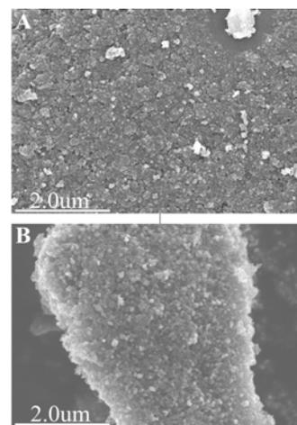
FIG. 2 Typical SEM images of the Fe<sub>3</sub>C@C samples obtained at 700 °C from (A) Fe<sub>3</sub>O<sub>4</sub> and (B) natural magnetite.
