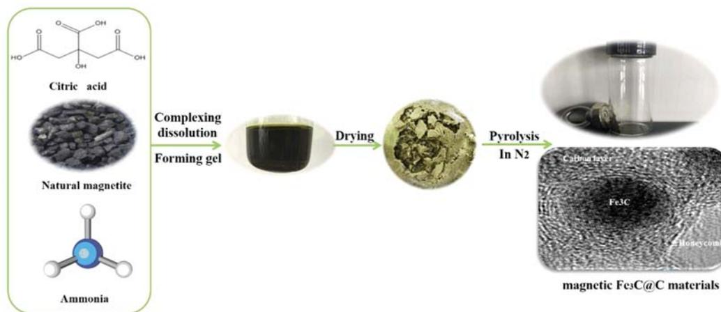
FIG. 5 Schematic of the synthesis process of the Fe<sub>3</sub>C@C samples modified by sol-gel method.
