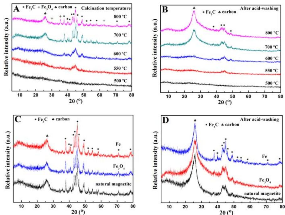
FIG. 1 XRD patterns of the  $\text{Fe}_3\text{C}@C$  samples from (A)  $\text{Fe}_3\text{O}_4$  and (B) after acid-treatment, and (C, D) from different iron sources with (D) after acid-treatment calcined at  $700^\circ\text{C}$ .
