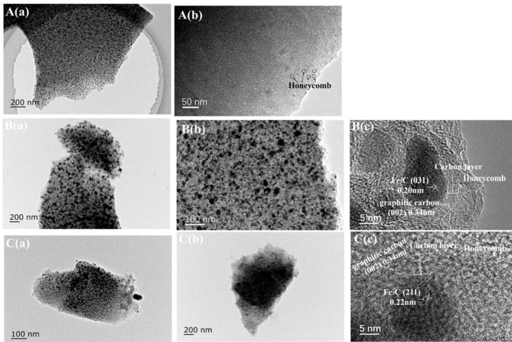
FIG. 3 TEM images of the  $\text{Fe}_3\text{C}@C$  samples obtained at  $500\text{ }^\circ\text{C}$  from  $\text{Fe}_3\text{O}_4$  A(a) before and A(b) after acid-treatment, at  $700\text{ }^\circ\text{C}$  from  $\text{Fe}_3\text{O}_4$ ; B(a) before, B(b) and B(c) after acid washing, at  $700\text{ }^\circ\text{C}$  with natural magnetite; C(a) before, C(b) and C(c) after acid washing.
