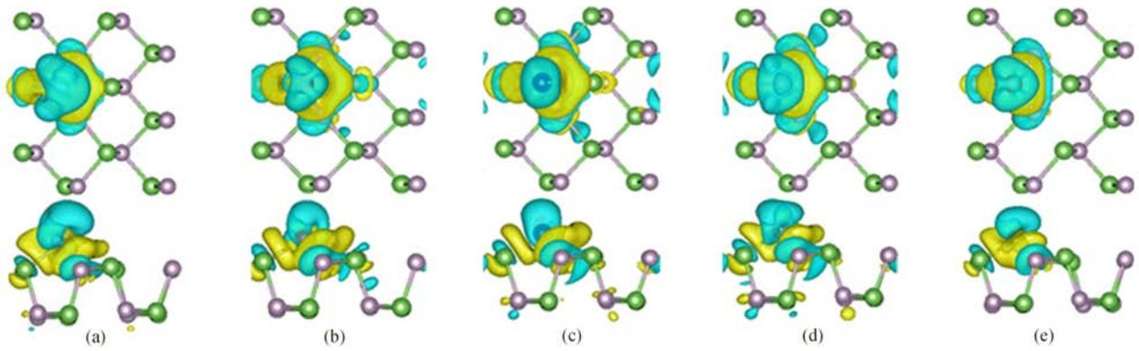
FIG. 5 The charge density difference of single (a) Ti, (b) V, (c) Cr, (d) Mn, (e) Fe adsorbed on the AsP monolayer.
