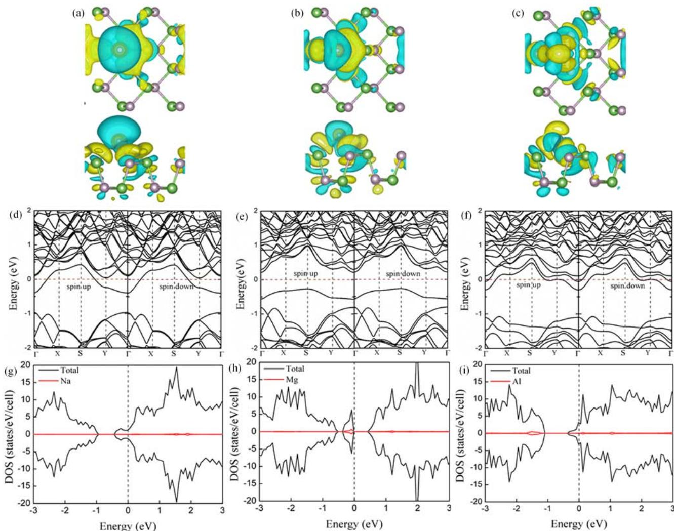
FIG. 4 The charge density difference of single (a) Na, (b) Mg, and (c) Al adsorbed on the AsP monolayer; the band structure of (d) Na-, (e) Mg-, and (f) Al-adsorbed AsP; the PDOS of (g) Na-, (h) Mg-, and (i) Al-adsorbed AsP.
