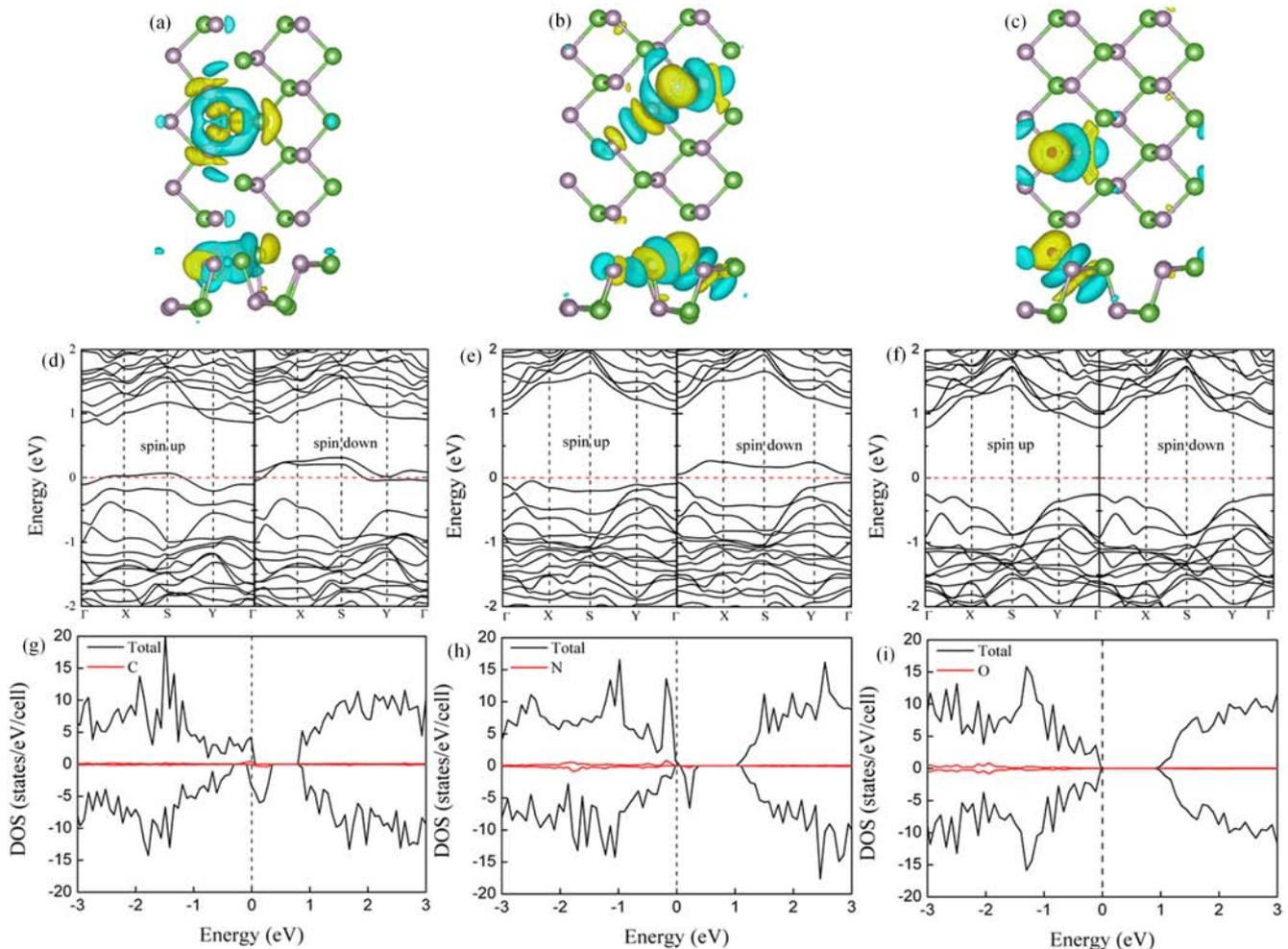
FIG. 3 The charge density difference of single (a) C, (b) N, and (c) O adsorbed on the AsP monolayer; the band structure of (d) C-, (e) N-, and (f) O-adsorbed AsP; the PDOS of (g) C-, (h) N-, and (i) O-adsorbed AsP.
