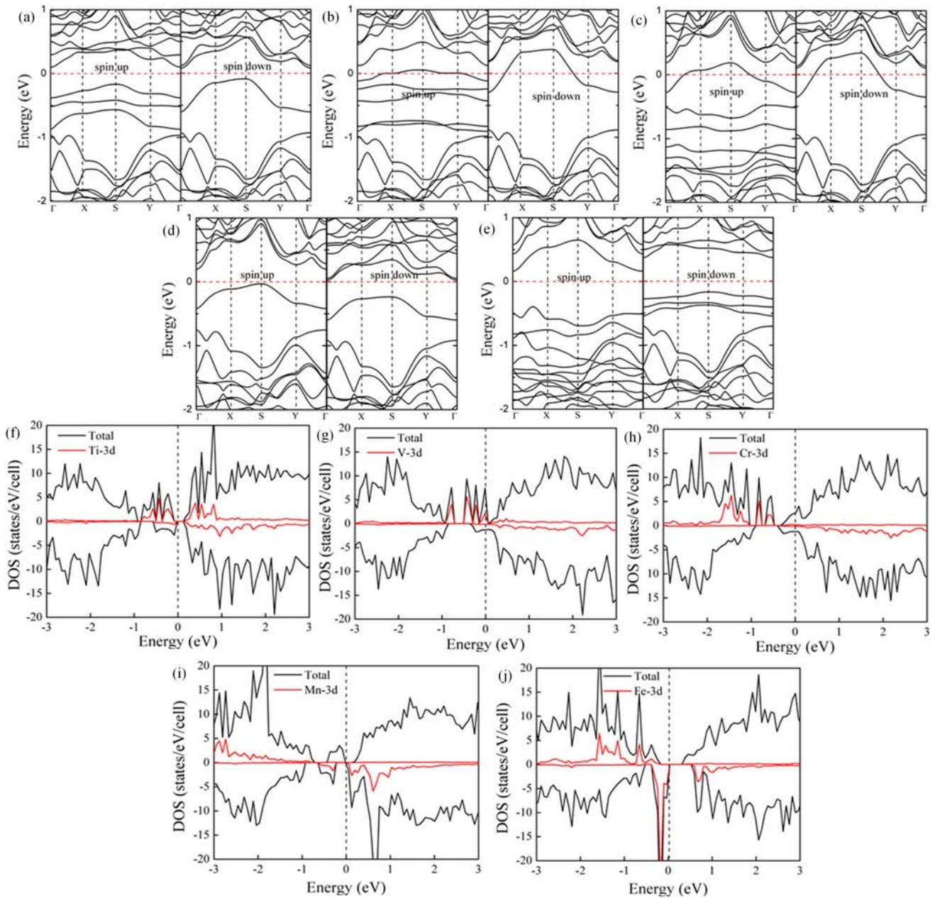
FIG. 6 The band structure of (a) Ti-, (b) V-, (c) Cr-, (d) Mn-, (e) Fe- adsorbed AsP; the PDOS of (f) Ti-, (g) V-, (h) Cr-, (i) Mn-, and (j) Fe-adsorbed AsP.
