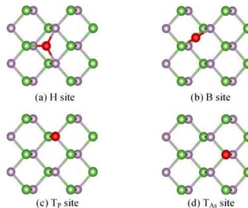
FIG. 2 Typical adatom adsorption sites on AsP monolayer: (a) H, (b) B, (c)  $T_P$ , and (d)  $T_{As}$ .
