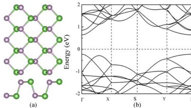
FIG. 1 (a) Illustration of top and side view of AsP monolayer. (b) Electronic band structure of pristine AsP.
