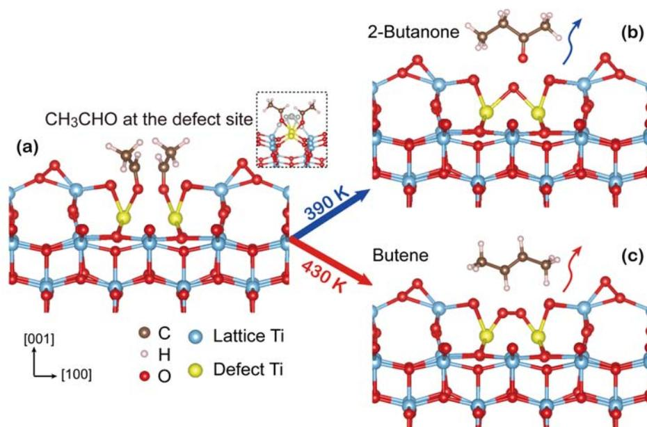
FIG. 4 Schematic drawings of (a) adsorption of paired CH<sub>3</sub>CHO at the reduced Ti<sub>4c</sub> pair, (b) production of 2-butanone by leaving one O atom at the defect site, and (c) production of butene by leaving two O atoms at the defect site. The inset shows the side view of (a).
