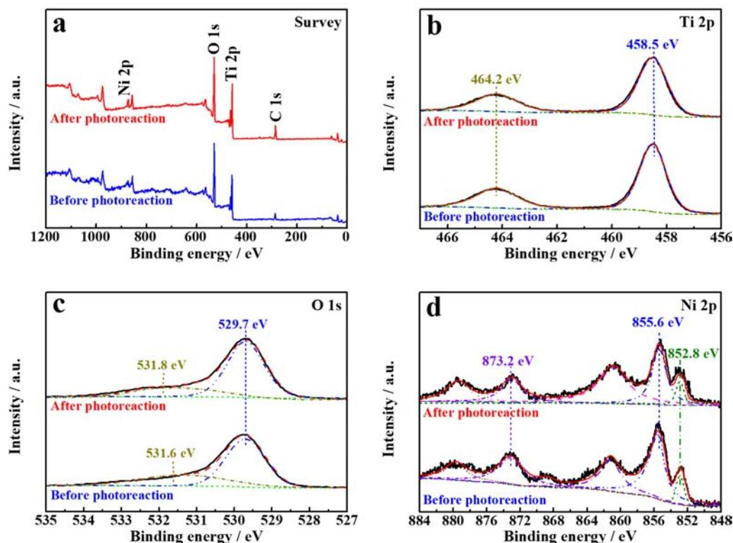
FIG. 2 (a) Survey, (b) Ti2p, (c) O1s, and (d) Ni2p XPS spectra of 1.0%Ni/BTN composite and its recycled product after the 12 h photoreaction.
