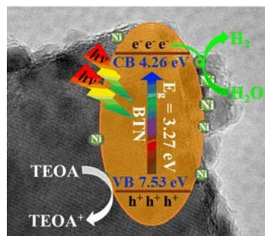
FIG. 8 The possible photocatalytic mechanism for  $H_2$  evolution over the Ni/BTN composite.
