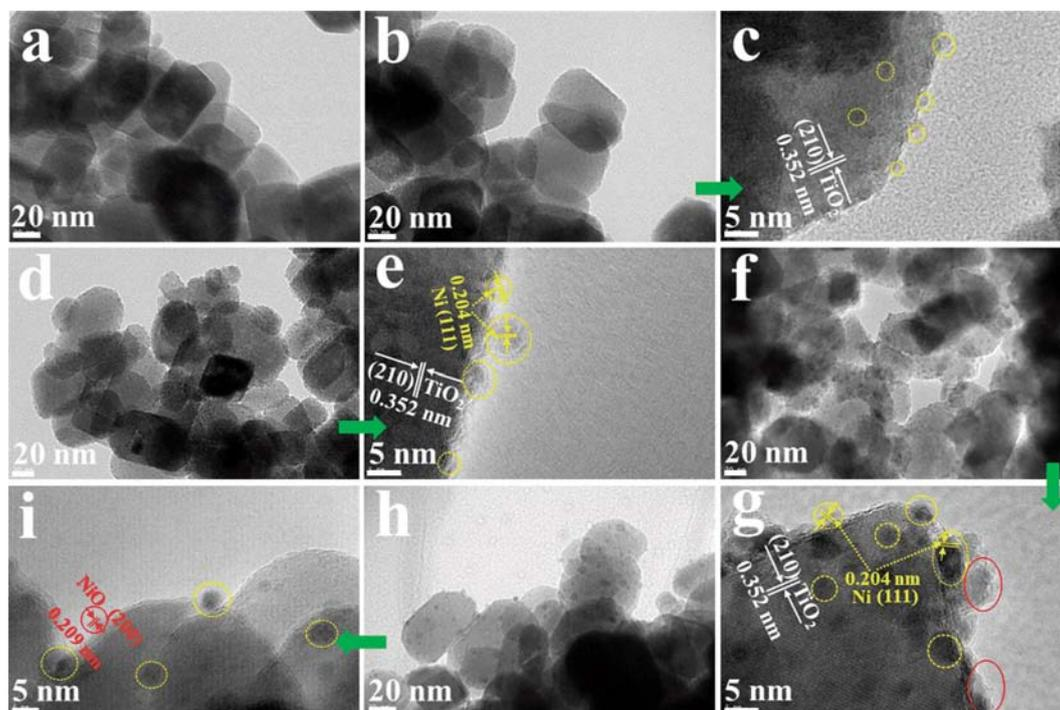
FIG. 4 TEM and HRTEM images of (a) the pristine BTN, (b, c) 1.0%Ni/BTN, (d, e) 5.0%Ni/BTN, (f, g) 10%Ni/BTN and (h, i) 10%Ni/BTN calcined at 200 °C for 2 h under Ar atmosphere.
