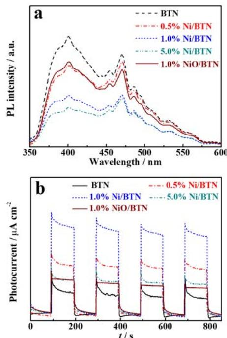
FIG. 9 (a) Photoluminescence spectra of the pristine BTN, NiO/BTN and Ni/BTN composites under excitation wavelength of 290 nm. (b) Photocurrent-time curves of the pristine BTN, NiO/BTN and Ni/BTN composites in NaOH solution under 300 W Xe-lamp irradiation.
