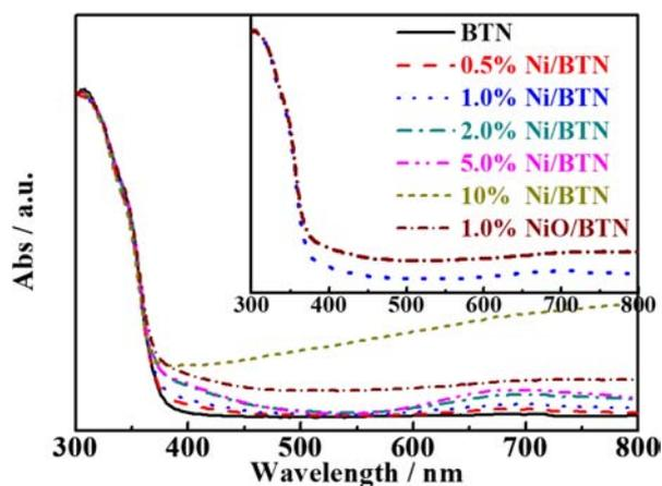
FIG. 5 UV-Vis diffuse reflectance absorption spectra of the pristine BTN and its Ni-loaded products (Ni/BTN) with different Ni-loading contents.
