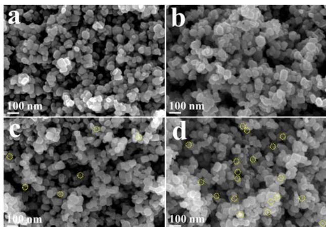
FIG. 3 FESEM images of (a) the pristine BTN, (b) 1.0%Ni/BTN, (c) 5.0%Ni/BTN, and (d) 10%Ni/BTN.
