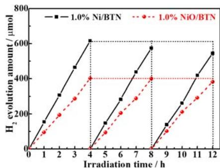
FIG. 7 Typical time course for  $H_2$  evolution over 1.0%Ni/BTN and 1.0%NiO/BTN composites under 300 W Xe-lamp irradiation. Conditions: 10 mg photocatalysts in 10 vol.% TEOA solution (10 mL, pH=6.00).
