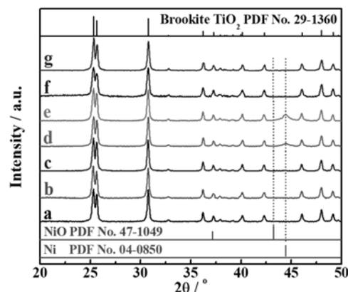
FIG. 1 XRD patterns of (a) the pristine BTN, (b) 0.5%Ni/BTN, (c) 1.0%Ni/BTN, (d) 5.0%Ni/BTN, (e) 10%Ni/BTN, (f) 1.0%NiO/BTN, and (g) 5.0%NiO/BTN.
