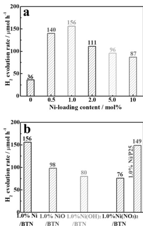
FIG. 6 (a) Photocatalytic H<sub>2</sub> evolution activity of Ni/BTN composites with various Ni-loading contents. (b) Comparison of photocatalytic H<sub>2</sub> evolution activities of various 1.0%Ni-containing cocatalyst-loaded BTN composites and the 1.0%Ni-loaded P25. Conditions: 10 mg catalyst in 10 vol.% TEOA solution (10 mL, pH=6.00) if otherwise stated.
