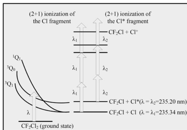
FIG. 4 Schematic potential energy surfaces illustrating the photodissociation of  $\text{CF}_2\text{Cl}_2$  around 235 nm.
