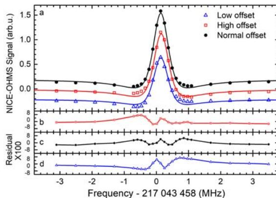
FIG. 4 Spectra of the R(4) line of  $\text{C}_2\text{H}_2$  recorded at different offsets applied in the NICE-OHMS measurements.
