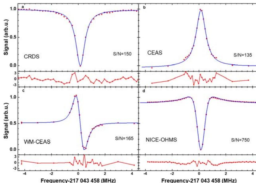
FIG. 2 Saturation spectrum of the R(4) line of  $C_2H_2$  near  $7239.79\text{ cm}^{-1}$  recorded by (a) CRDS, (b) CEAS, (c) wavelength-modulated CEAS ( $1f$ ), and (d) wavelength-modulated NICE-OHMS ( $1f$ ). The sample pressure was 1.3 Pa. Fitting residuals were multiplied by a factor of 100.
