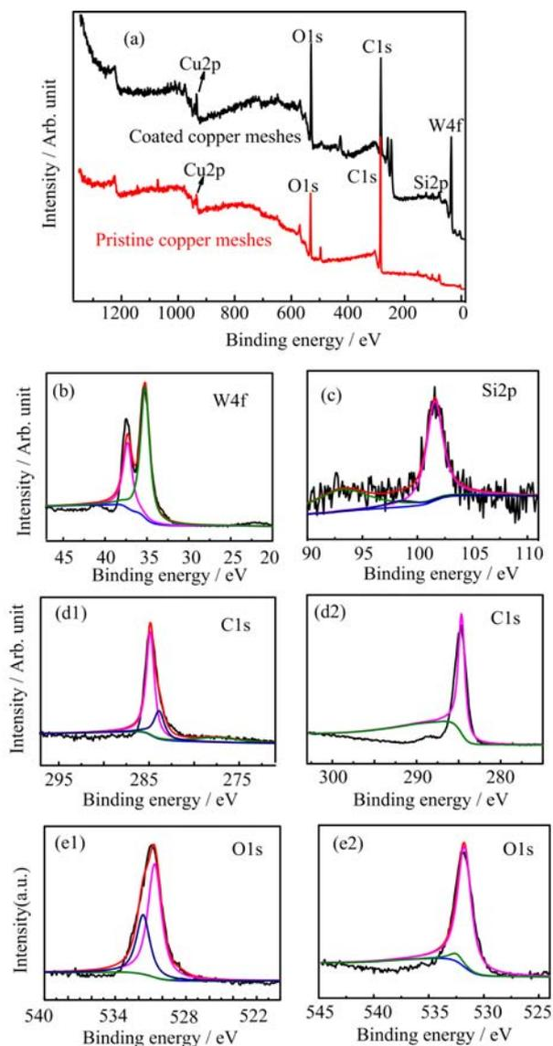
FIG. 4 (a) XPS survey spectra of pristine and coated copper mesh. (b) W 4f high-resolution spectra of coated copper mesh. (c) Si 2p high-resolution spectra of coated copper mesh. (d) and (e) show C 1s and O 1s high-resolution spectra of coated (d1, e1) and pristine (d2, e2) copper mesh.
