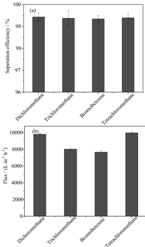
FIG. 6 Experiments of oil/water separation. (a) Separation efficiency of various heavy oil/water mixtures through coated copper mesh. (b) Flux of various oil/water mixtures through coated copper mesh.
