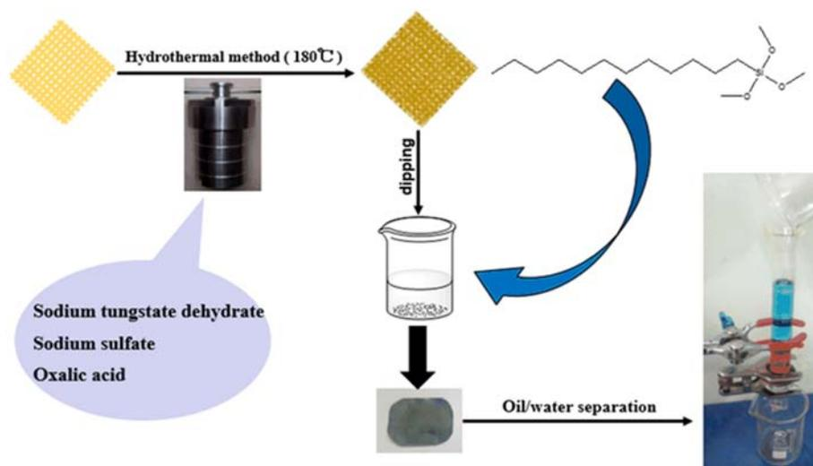
FIG. 1 Schematic description of the preparation for DTMS@WO<sub>3</sub> coated copper mesh.
