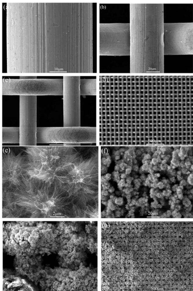
FIG. 2 (a–d) SEM images of pristine copper mesh. (e–h) SEM images of coated copper mesh.
