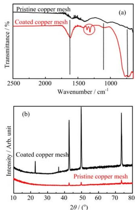
FIG. 3 (a) FT-IR spectra of pristine copper mesh and the coated copper mesh. (b) XRD patterns for pristine copper mesh and the coated copper mesh.
