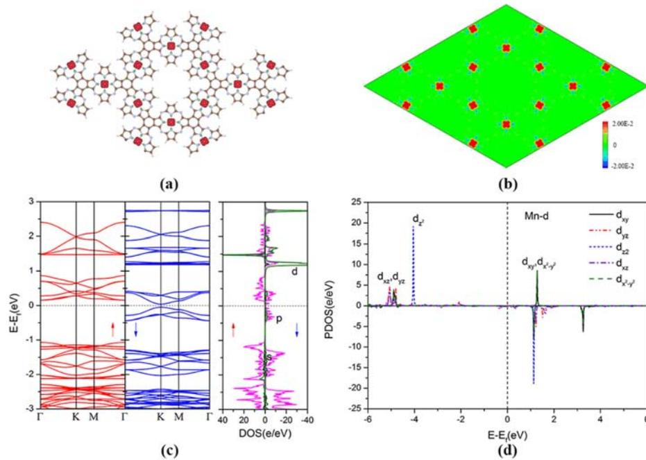
FIG. 2 (a) Isosurfaces at the value  $0.01 \text{ e}/\text{\AA}^3$  and (b) 2D slice of spin-polarized electron density for a  $2 \times 2$  supercell of the 2D FM kag-MnPc framework. (c) Band structure and corresponding PDOS of s (black), p (pink), and d (green) orbitals in the 2D FM kag-MnPc framework. (d) PDOS of the five d orbitals in the 2D FM kag-MnPc framework.
