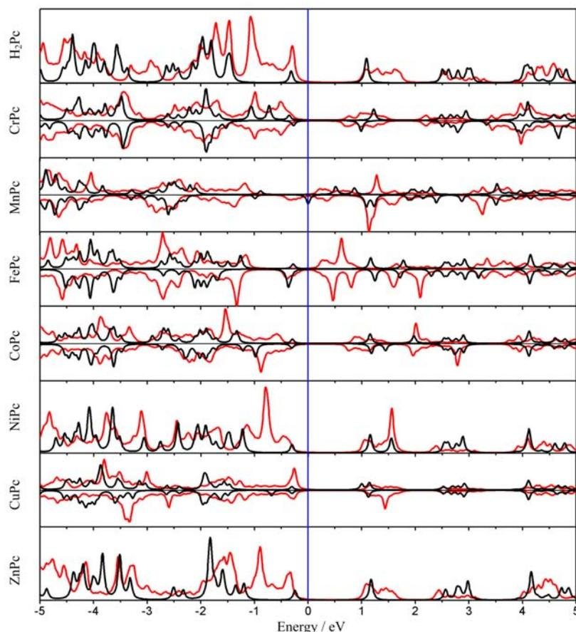
FIG. 6 Electronic DOS for the H<sub>2</sub>Pc/TMPc molecules (black lines) and corresponding kag-H<sub>2</sub>Pc/TMPc frameworks (red lines). The Fermi energy is shifted to zero and marked by the blue line.
