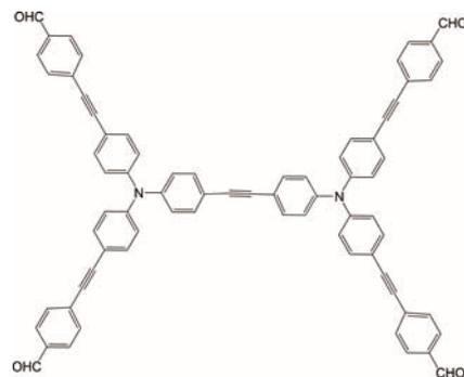
FIG. 6 The geometric structure of compound Mol.4.
