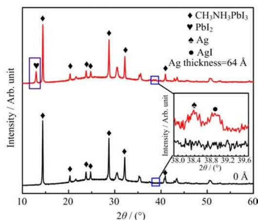
FIG. 2 The XRD patterns of the pristine  $\text{CH}_3\text{NH}_3\text{PbI}_3$  sample and the sample deposited with 64 Å thick Ag. The inset is the partially enlarged view of the XRD pattern (from  $37.9^\circ$  to  $39.7^\circ$ ). The characteristic peaks at  $2\theta=38.35^\circ$  and  $38.95^\circ$  correspond to metallic Ag and AgI species, respectively. The peak at  $2\theta=12.89^\circ$  corresponds to  $\text{PbI}_2$  species.
