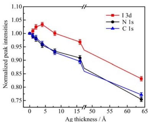
FIG. 4 The evolution of peak intensities of C 1s, N 1s, and I 3d spectra as a function of Ag thickness on the  $\text{CH}_3\text{NH}_3\text{PbI}_3$  surface. The break region of the horizontal axis is from 17 Å to 48 Å. All the peak intensities are normalized to those from the pristine  $\text{CH}_3\text{NH}_3\text{PbI}_3$  surface.
