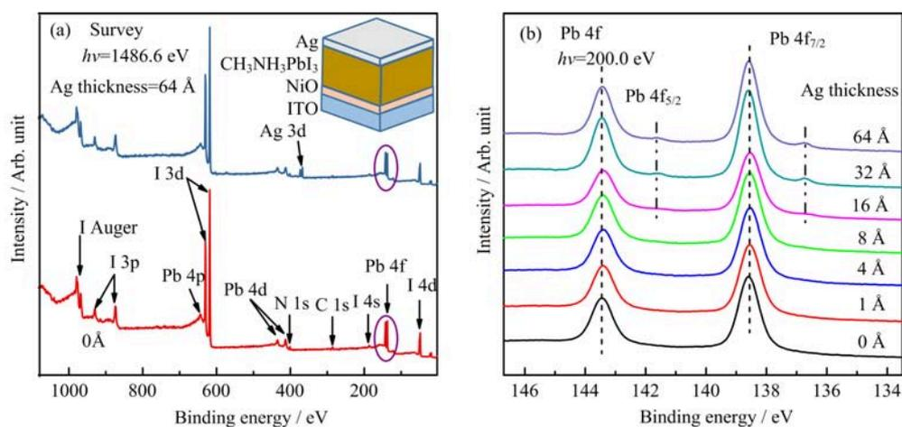
FIG. 1 (a) XPS survey spectra of the pristine  $\text{CH}_3\text{NH}_3\text{PbI}_3$  layer (red curve) and the sample deposited with 64 Å of Ag (blue curve). The inset shows the schematic architecture of the sample ITO/NiO/ $\text{CH}_3\text{NH}_3\text{PbI}_3$ /Ag. (b) The evolution of Pb 4f XPS as a function of the Ag thickness.
