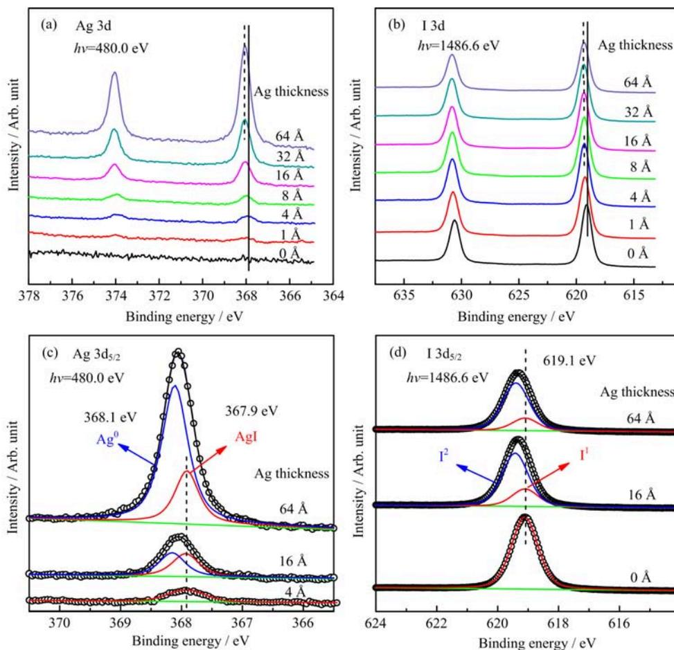
FIG. 3 The evolution of (a) Ag 3d, (b) I 3d core-level spectra as a function of the Ag thickness. Representative peak fitting results of (c) Ag  $3d_{5/2}$  and (d) I  $3d_{5/2}$  for Ag deposition on perovskite surface with different thicknesses.
