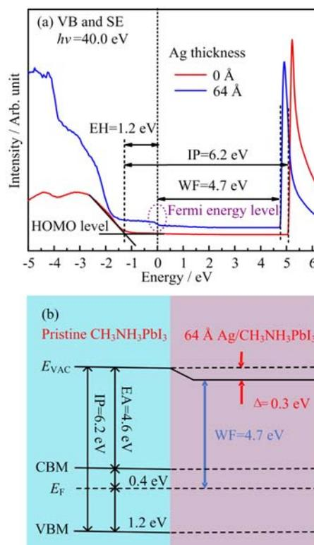
FIG. 5 (a) Thickness dependent UPS spectra of Ag on  $\text{CH}_3\text{NH}_3\text{PbI}_3$  coated on the NiO/ITO substrate including the secondary cut-off region and the valence band edge region. (b) The schematic drawing of the energy level alignment diagram at the  $\text{CH}_3\text{NH}_3\text{PbI}_3/\text{Ag}$  interface. IP is the ionization potential, EA is the electron affinity, EH is the hole transport barrier, WF is the work function, and  $\Delta$  is the interfacial dipole.
