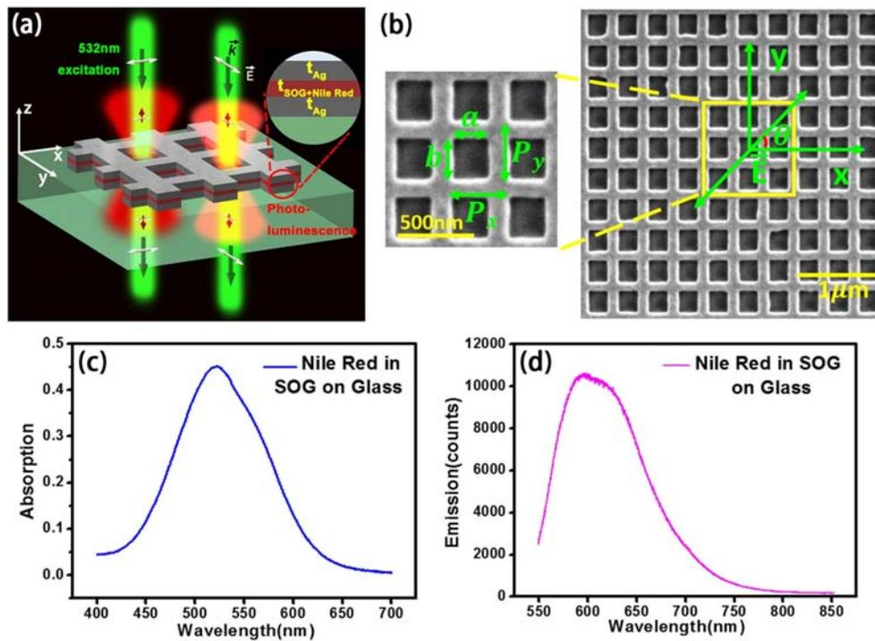
FIG. 1 MDM fishnet material. (a) Schematic of the fishnet structure. (b) Scanning electron microscopy image of the fabricated structure. (c) Absorption and (d) photoluminescence emission spectra of Nile Red molecules mixed in SOG solution and then spin-coated on glass substrate.
