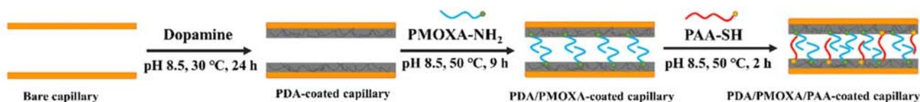
Scheme 1 The procedure of PDA/PMOXA/PAA coating grafted onto the fused-silica capillary inner wall.
