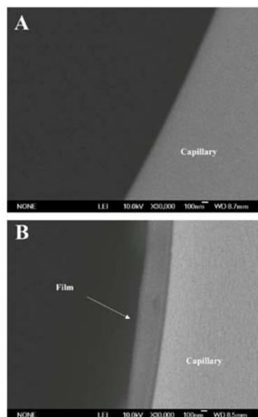
FIG. 1 SEM images of bare (A) and PDA/PMOXA/PAA (B) coated capillary with the magnification of  $\times 30000$ .
