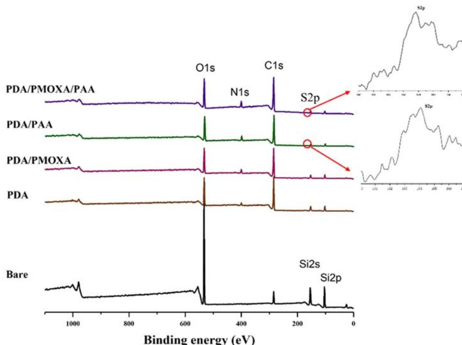
FIG. 2 XPS spectra of wide scan for the bare, PDA, PDA/PMOXA, PDA/PAA, and PDA/PMOXA/PAA coated capillary raw materials.
