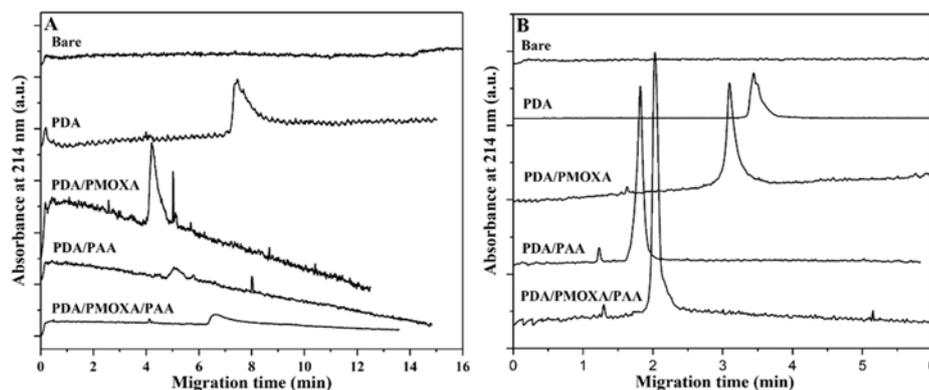
FIG. 5 Separation of BSA (0.5 mg/mL) in the bare and polymer coated capillaries at pH=5.0 ( $I=10^{-5}$  mol/L) (A) and separation at pH=9.0 ( $I=0.1$  mol/L) (B) in CE. Experimental conditions: temperature of 25 °C, injection of 5.0 s at 0.5 psi, separation voltage of 15 kV, detection of 214 nm.
