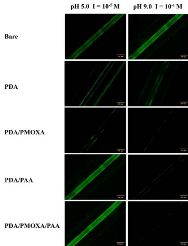
FIG. 3 Fluorescence microscope images of bare, and PDA, PDA/PMOXA, PDA/PAA, and PDA/PMOXA/PAA coated capillaries after adsorption of FITC-BSA solution (pH=5.0 and  $I=10^{-5}$  mol/L, 1.0 mg/mL) and images of corresponding capillaries after rinse using the phosphate buffer solution (pH=9.0 and  $I=10^{-1}$  mol/L). The scale bar is 100  $\mu\text{m}$ .
