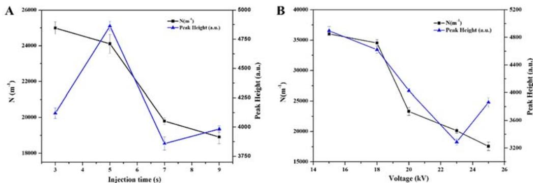
FIG. 4 Effects of CE conditions with on-line preconcentration procedure of standard BSA solution (0.5 mg/mL) using PDA/PMOXA/PAA coated capillary at pH=9.0 ( $I=0.1$  mol/L) ( $n=5$ ). (A) The effect of injection time, (B) the effect of separation voltage. Experimental conditions: temperature of 25 °C, detection of 214 nm.
