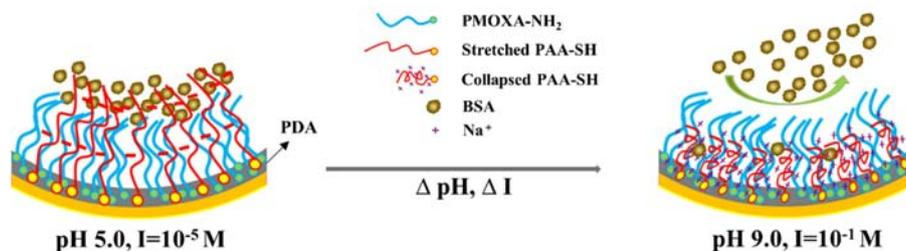
Scheme 2 Mechanism of adsorption and desorption of BSA on the PDA/PMOXA/PAA coated capillary.
