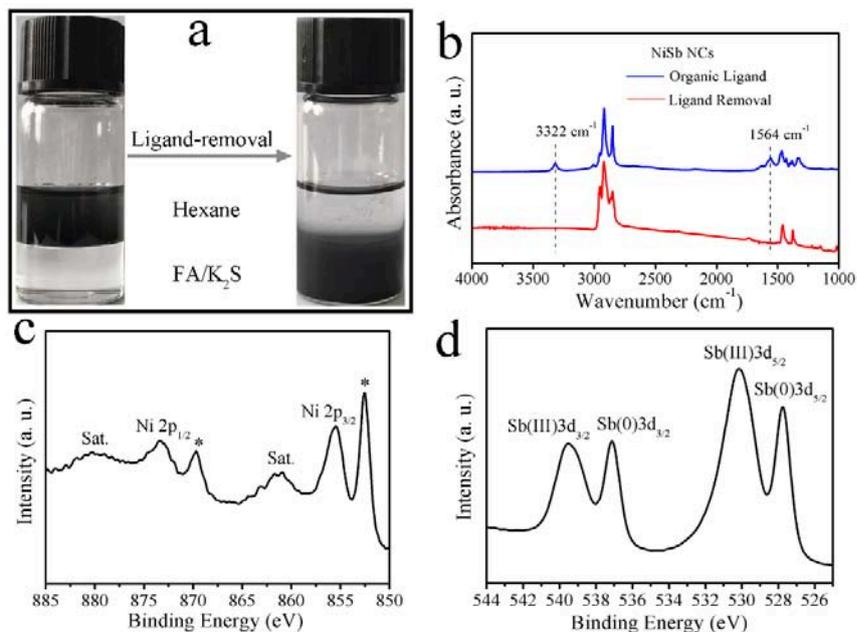
FIG. 3 (a) Photographs illustrating phase transfer of NiSb nanoparticles from hexane to formamide, (b) ATR-FTIR spectra of the as-obtained NiSb nanoparticles, blue and red curves refer to the results of the sample before and after phase transfer, (c) XPS spectrum of Ni 2p, and (d) XPS spectrum of Sb 3d in NiSb nanoparticles.
