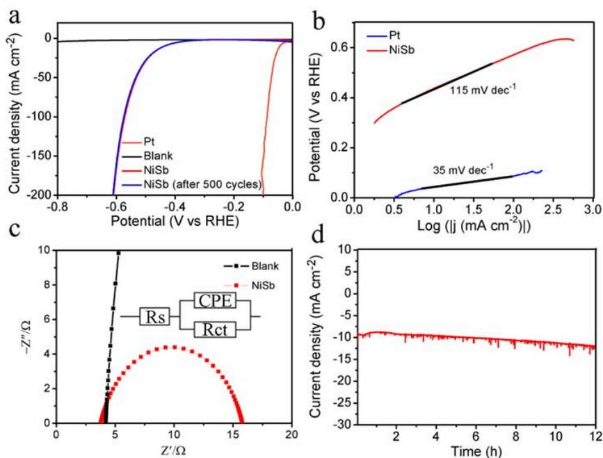
FIG. 4 (a) Polarization curves and (b) Tafel slopes of the as-prepared NiSb nanoparticles electrocatalyst, (c) EIS at the overpotential of 700 mV, and (d) time-dependent current density curve of the as-prepared NiSb nanoparticles electrocatalyst.
