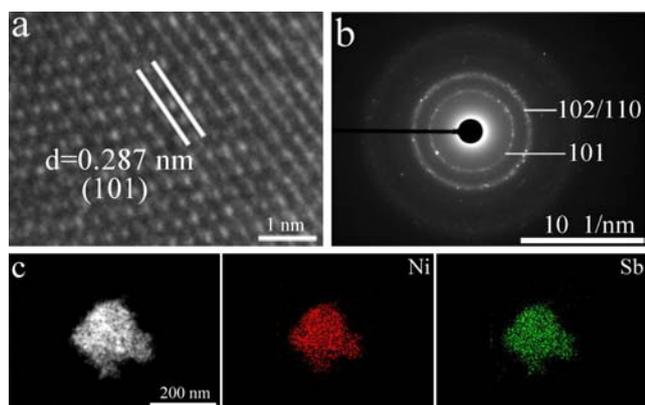
FIG. 2 (a) HRTEM image of the NiSb nanoparticles, (b) SAED pattern and (c) HAADF-STEM image, STEM-EDX elemental mappings of Ni and Sb.
