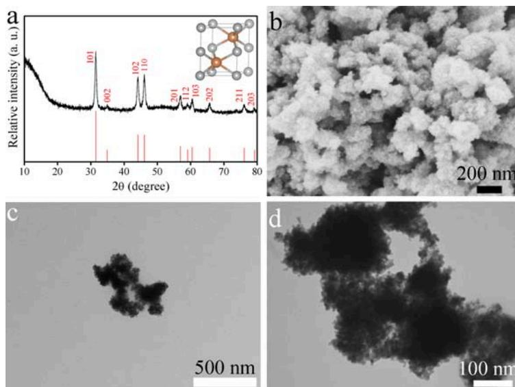
FIG. 1 (a) XRD pattern of the as-synthesized NiSb nanoparticles along with the corresponding standard pattern of hexagonal NiSb (JCPDS card No.03-065-4339), and the inset is schematic representation of the NiSb crystal structure, (b) SEM image, (c) low- and (d) high-magnification TEM images for the NiSb nanoparticles.
