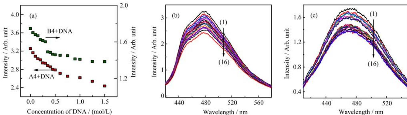
FIG. 6 (a) Fluorescence intensity of polymer A4 and B4 with the different concentration of DNA. Fluorescence intensity spectra of A4 (b) and B4 (c) the different concentration of DNA with 0 (1), 0.05 (2), 0.1(3), 0.15 (4), 0.2 (5), 0.25 (6), 0.3 (7), 0.35 (8), 0.4 (9), 0.45 (10), 0.5 (11), 0.6 (12), 0.75 (13), 1.0 (14), 1.25 (15), 1.5 mol/L (16).
