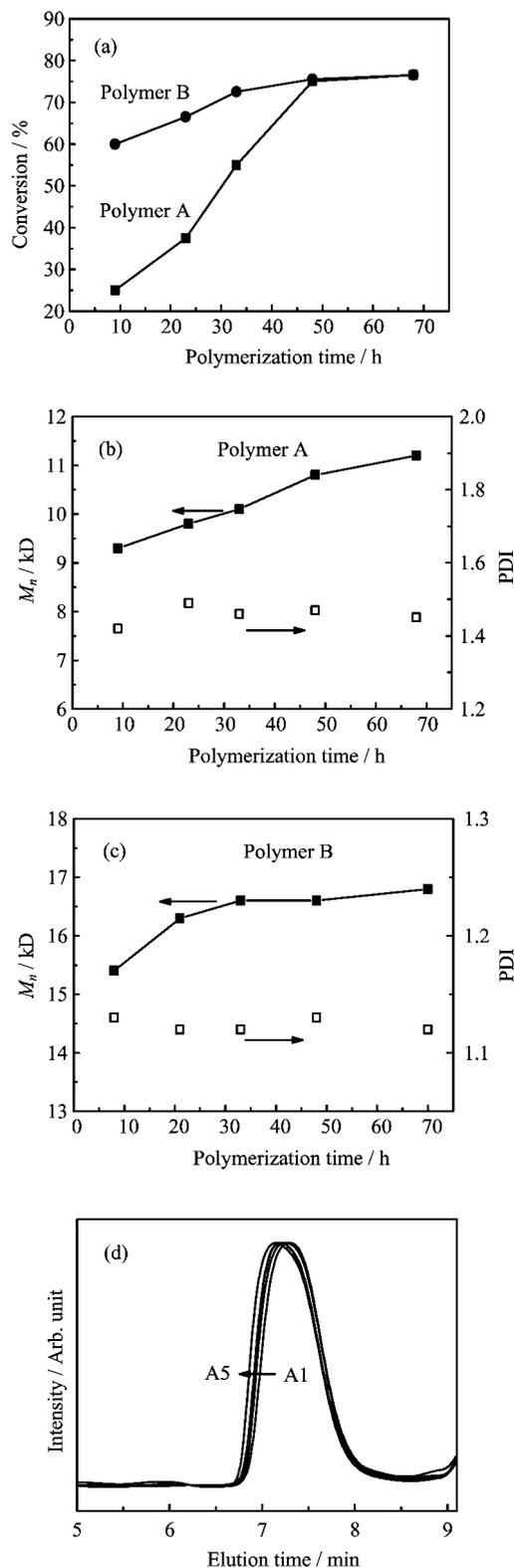
FIG. 3 Dependence of conversion (a), molecular weight and PDI of polymers A (b) and B (c) on polymerization time with [MTDA]/[CTA]/[AIBN]=100/3/1. (d) GPC traces of polymers of A1–A5.
