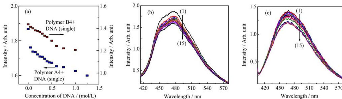
FIG. 7 (a) Fluorescence intensity of polymer A4 and B4 with the different concentration of single DNA. Fluorescence intensity spectra of A4 (b) and B4 (c) with the concentration single DNA with 0 (1), 0.05 (2), 0.1(3), 0.15 (4), 0.2 (5) 0.25 (6), 0.3 (7), 0.35 (8), 0.4 (9), 0.45 (10), 0.5 (11), 0.6 (12), 0.75 (13), 1.0 (14), 1.25 mol/L (15).
