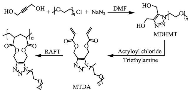
Scheme 1 Synthesis of the macromonomer MTDA and cyclopolymerization of the macromonomer MTDA.
