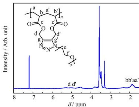
FIG. 4  $^1\text{H}$  NMR spectrum of cyclopolymer in  $\text{CDCl}_3$ .
