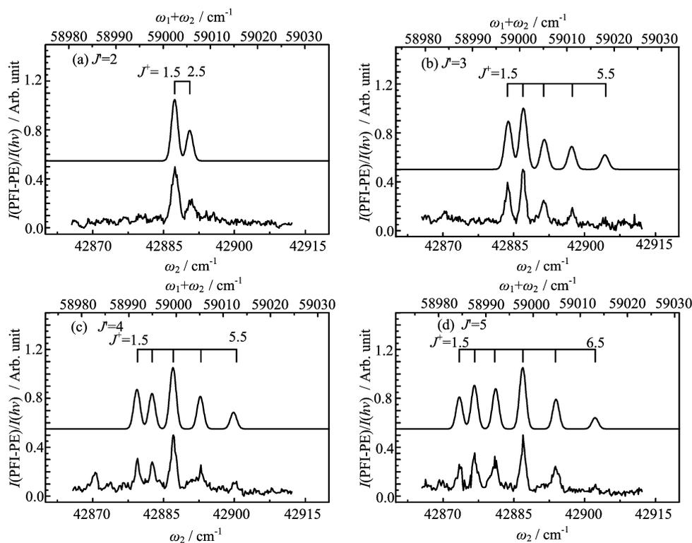
FIG. 8 Rotationally resolved PFI-PE spectra (lower) and the simulated spectra (upper) for the formation of  $\text{VN}^+(X^2\Delta_{3/2}, v^+=2, J^+)$  from the rotational levels, (a)  $J'=2$ , (b)  $J'=3$ , (c)  $J'=4$ , and (d)  $J'=5$ , of the intermediate  $\text{VN}^*(D^3\Pi_0, v'=0)$  state.
