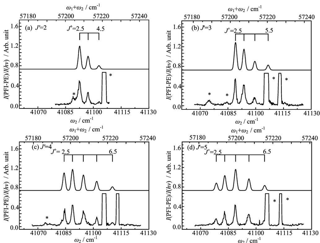
FIG. 5 Rotationally resolved PFI-PE spectra (lower) and the simulated spectra (upper) for the formation of  $\text{VN}^+(X^2\Delta_{5/2}, v^+=0, J^+)$  from the rotational levels, (a)  $J'=2$ , (b)  $J'=3$ , (c)  $J'=4$ , and (d)  $J'=5$ , of the intermediate  $\text{VN}^*(D^3\Pi_0, v'=0)$  state.
