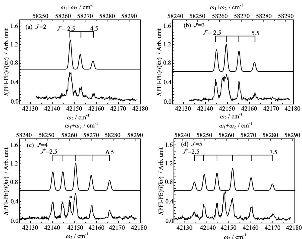
FIG. 7 Rotationally resolved PFI-PE spectra (lower) and the simulated spectra (upper) for the formation of  $\text{VN}^+(X^2\Delta_{5/2}, v^+=1, J^+)$  from the rotational levels, (a)  $J'=2$ , (b)  $J'=3$ , (c)  $J'=4$ , and (d)  $J'=5$ , of the intermediate  $\text{VN}^*(D^3\Pi_0, v'=0)$  state.
