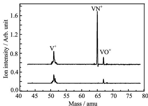
FIG. 2 The upper spectrum is the TOF mass spectrum for  $V^+$ ,  $VN^+$  and  $VO^+$  observed by means of two-color VIS-UV resonance enhanced photoionization scheme with VIS  $\omega_1$  fixed at  $16113.88\text{ cm}^{-1}$  and UV  $\omega_2$  fixed at  $47619\text{ cm}^{-1}$ . The lower spectrum was recorded by means of one-color UV multi-photon ionization scheme, *i.e.*, the VIS  $\omega_1$  laser beam was turned off and only the UV  $\omega_2$  laser was turned on.
