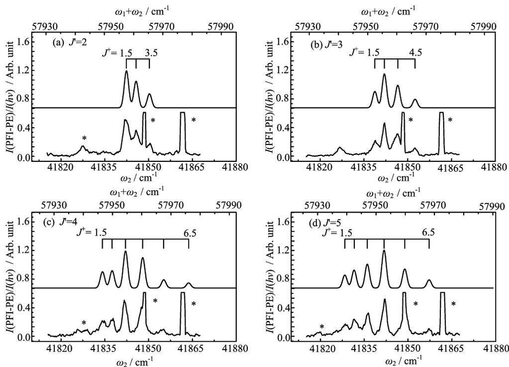
FIG. 6 Rotationally resolved PFI-PE spectra (lower) and the simulated spectra (upper) for the formation of  $\text{VN}^+(X^2\Delta_{3/2}, v^+=1, J^+)$  from the rotational levels, (a)  $J'=2$ , (b)  $J'=3$ , (c)  $J'=4$ , and (d)  $J'=5$ , of the intermediate  $\text{VN}^*(D^3\Pi_0, v'=0)$  state.
