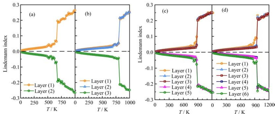
FIG. 2 The Lindemann index of each atomic layer as a function of temperature for the Au nanofilms with different thicknesses: (a) L2, (b) L3, (c) L5, and (d) L6 nanofilms.
