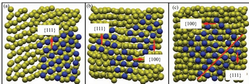
FIG. 5 The final configurations of (a) L3 nanofilm at 800 K, (b) L5 nanofilm at 880 K, and (c) L6 nanofilm at 940 K. The blue spheres represent the Au atoms in the outermost layer.
