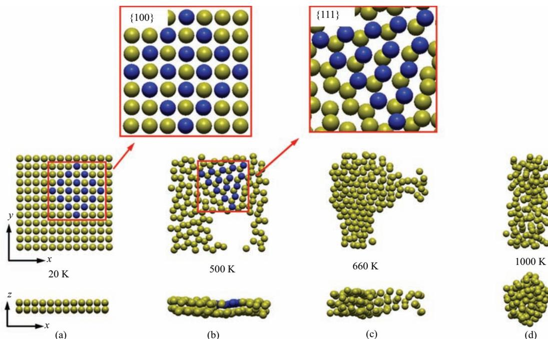
FIG. 4 The final configurations of L2 nanofilm at four typical temperatures. (a) 20 K, (b) 500 K, (c) 660 K, and (d) 1000 K. The blue spheres represent the Au atoms in the outermost layer.
