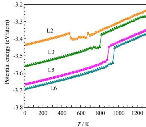
FIG. 1 The potential energy per atom as a function of temperature for the Au nanofilms with different thicknesses.
