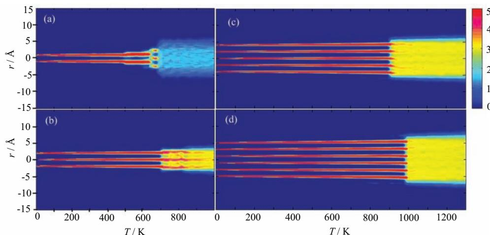
FIG. 3 The atomic number distribution perpendicular to the surface as a function of temperature for the Au nanofilms with different thicknesses: (a) L2, (b) L3, (c) L5, and (d) L6 nanofilms.
