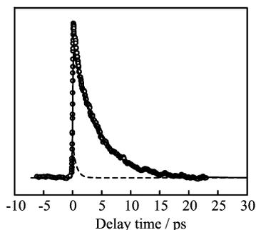
FIG. 1 Time-resolved total ion signals of parent ion as a function of delay time between the pump pulse at 267 nm and the probe pulse at 800 nm. The circles represent the experimental results, and the dash line and solid line represent the fitting results.
