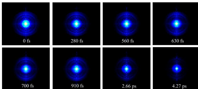
FIG. 3 A series of time-resolved BASEX-inverted photoelectron images of 2,6-dimethylpyridine observed using a pump laser wavelength of 267 nm and a probe wavelength of 800 nm. The linear polarizations of the pump and probe lasers are aligned vertical in the plane of the figure.
