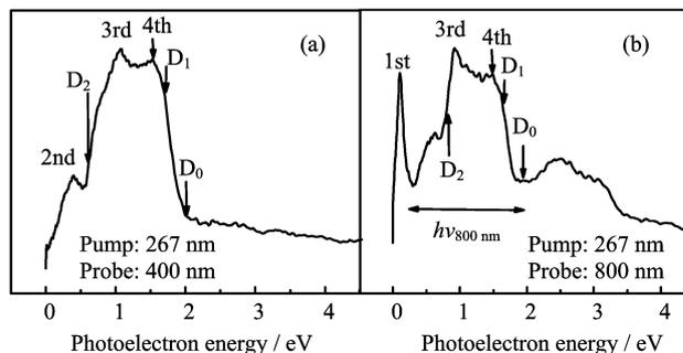
FIG. 2 PKE distributions extracted from the image at  $\Delta t=0$  for different probe wavelengths. (a) Two-photon absorption of 400 nm probe pulse. (b) Four-photon absorption of 800 nm probe pulse
