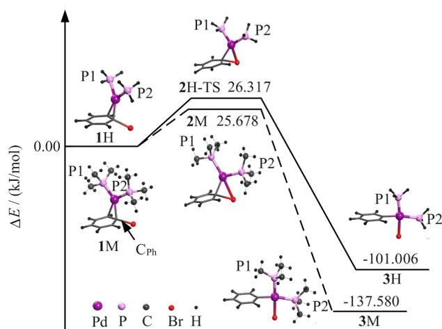
FIG. 3 Energy profile of Pd(PR<sub>3</sub>)<sub>2</sub> oxidative addition to bromobenzene (PR<sub>3</sub>=PH<sub>3</sub> (solid line) and PMe<sub>3</sub> (dashed line)). The energies were calculated in DMF solvent and given in kJ/mol.
