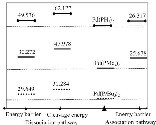
FIG. 5 Cleavage energy and the oxidative addition barrier energy of different diphosphine palladium and monophosphine palladium in DMF solvent in kJ/mol.
