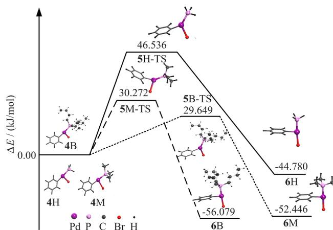
FIG. 4 Relative energy profile of PdPR<sub>3</sub> oxidative addition to bromobenzene (PR<sub>3</sub>=PH<sub>3</sub> (solid line), PMe<sub>3</sub> (dotted line), and PtBu<sub>3</sub> (dashed line)). The energies were calculated in DMF solvent and given in kJ/mol.
