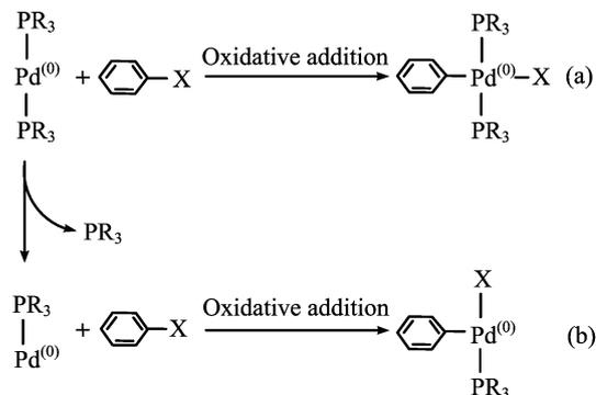
FIG. 6 Pathways of different size of ligand on the oxidative addition with bromobenzene. (a) For the less bulky phosphines, such as  $\text{PH}_3$  and  $\text{PMe}_3$ . (b) For the large bulky phosphines, such as  $\text{PtBu}_3$ .
